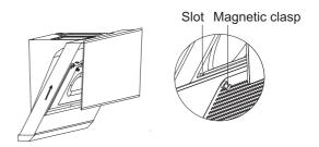
Hold the two magnetic clasps with slightly outward force to make the filter no longer been sucked. Then lift the filter screen as per the arrow direction to make it out of slot. At last, take the filter screen outward for cleaning.
