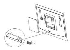
Push the light by hand from inside, and then disconnect the wire for repair and replacement.
