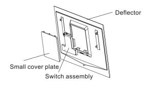
Take out the switch assembly and unplug the connection line for maintenance and replacement.
