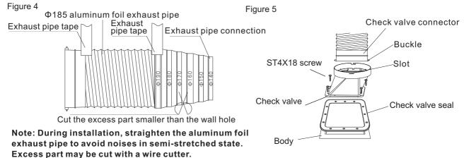
The exhaust wall hole diameter shall be close to that of the exhaust pipe, which shall not be too small. Otherwise, it will cause poor exhaust efficiency, more noises and lower airflow, etc. The connection between the pipe and the hole or the public flue must be sealed tightly to ensure that, the pipe and the check valve or public flue are connected securely. The blades at the check valve connection or public flue connection must be flexible.
