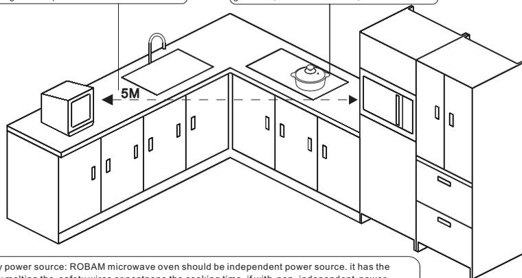
Electricity power source: ROBAM microwave oven should be independent power source, it has the possibility melting the safety wires or postpone the cooking time, if with non-independent power system. Don't use high power capacity safety wire.
