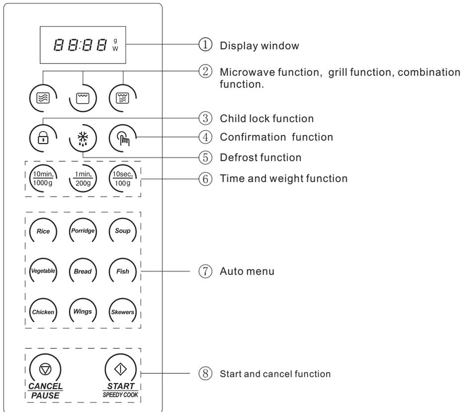
Note: the buttons on the panel outer ring can emit red light. Each button operation or the function running, the ring will light. The upper picture shows the aura and display all emitting mode.
