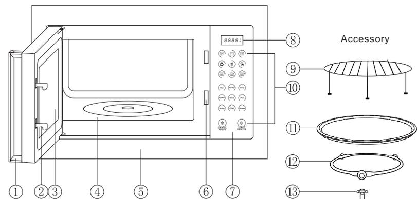
1. Handle    2. Door Latch    3. Door Screen    4. Cavity    5. Oven Front Plate
