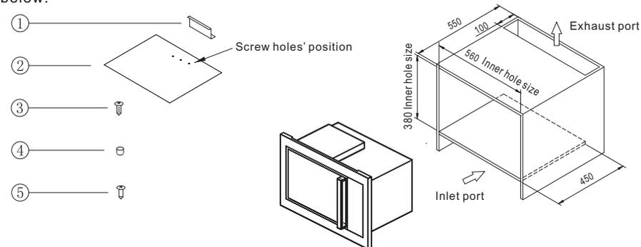
1. Positioning plate 2. Install paper 3. Screws 4x10(3pcs) 4. Screw cap 5. Screws 4x35(1pcs)
