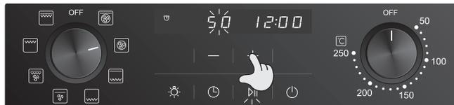
Adjust temperature: turn the temperature selector knob to adjust baking temperature (as shown below).
